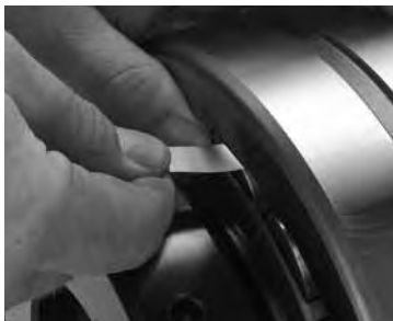
Fig. D-7. Measure RIC before installation.
