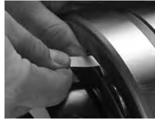
Fig. D-3. Measure RIC before installation.
